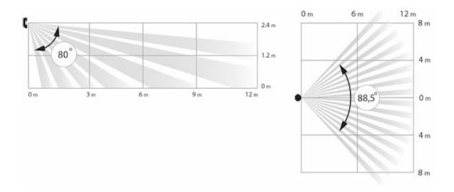
If the detector is not installed at the recommended height, this will reduce the area of the motion detection zone and impair the operation of the function of ignoring animals.
