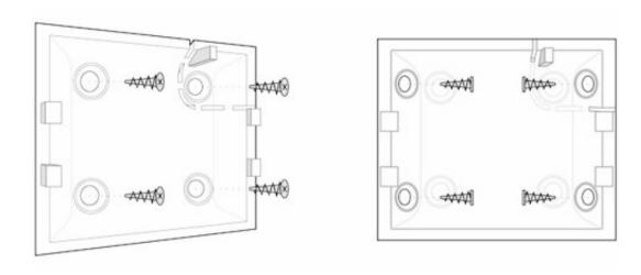
1. Attach the SmartBracket panel to the surface using bundled screws, using at least two fixing points (one of them – above the tamper). If you select other attachment hardware, make sure that they do not damage or deform the panel.
